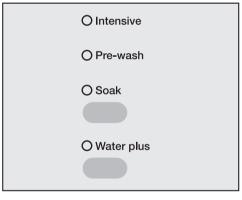
Press the appropriate additional option button. Press the top button repeatedly until the indicator light(s) for the additional option(s) you want comes on.
